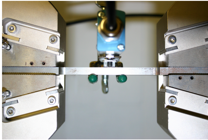
Figure 4.2: Experimental setup, showing the grip of the tensile test machine, the A36 test specimen, and the Barkhausen probe kept in a stable position by the clamp.
